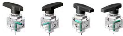
Ports 1 and 2 open Ports 1 and 3 open Ports 1 and 4 open Ports 1 and 5 open
